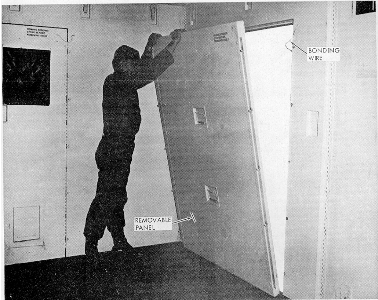
Figure 2-3(4). Interchanging removable panels and swinging door panels (Sheet 4 of 4).
