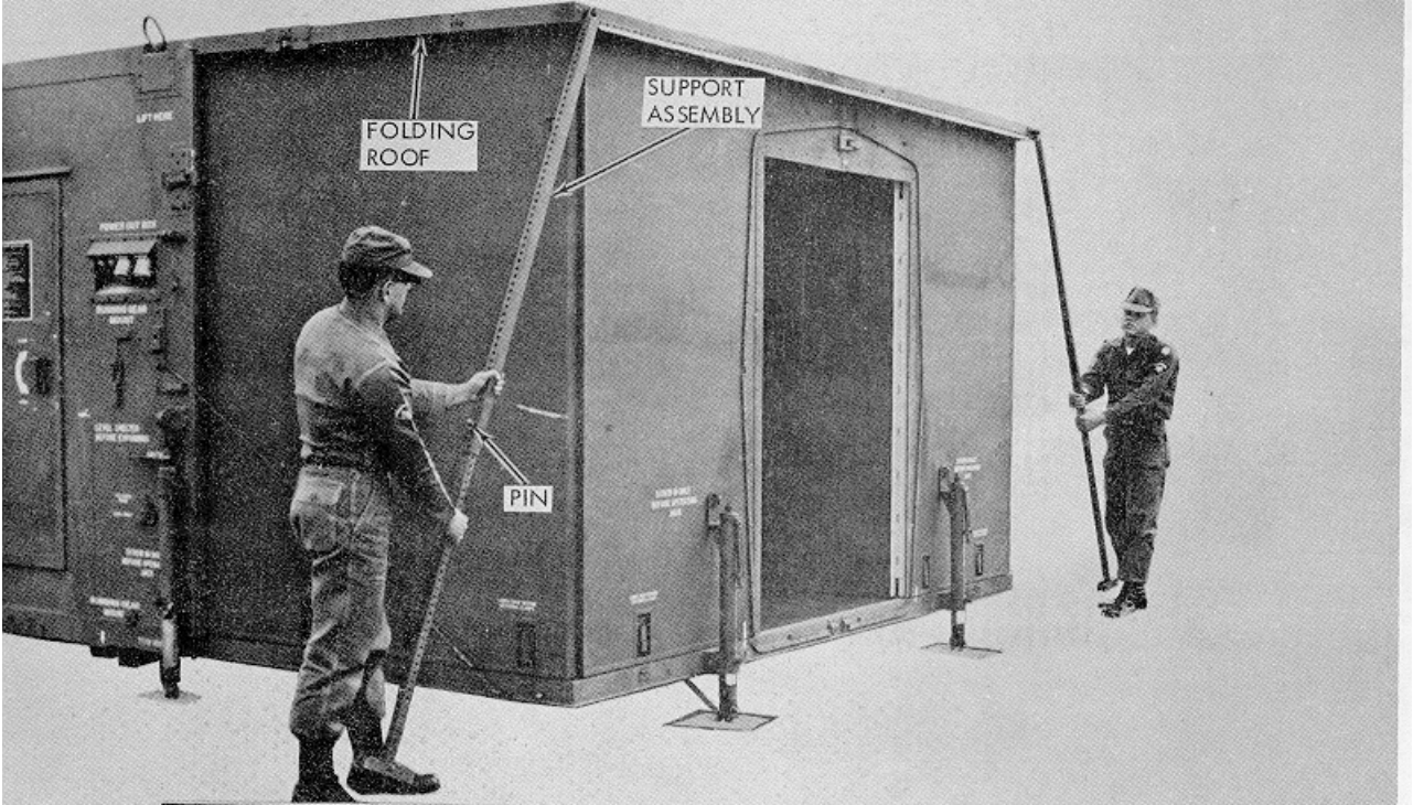
12 PULL SUPPORT ASSEMBLIES OUTWARD AND ALLOW FOLDING ROOF TO REST ON SHELTER. REMOVE PIN AND COLLAPSE SUPPORT ASSEMBLY. REINSTALL PIN.
