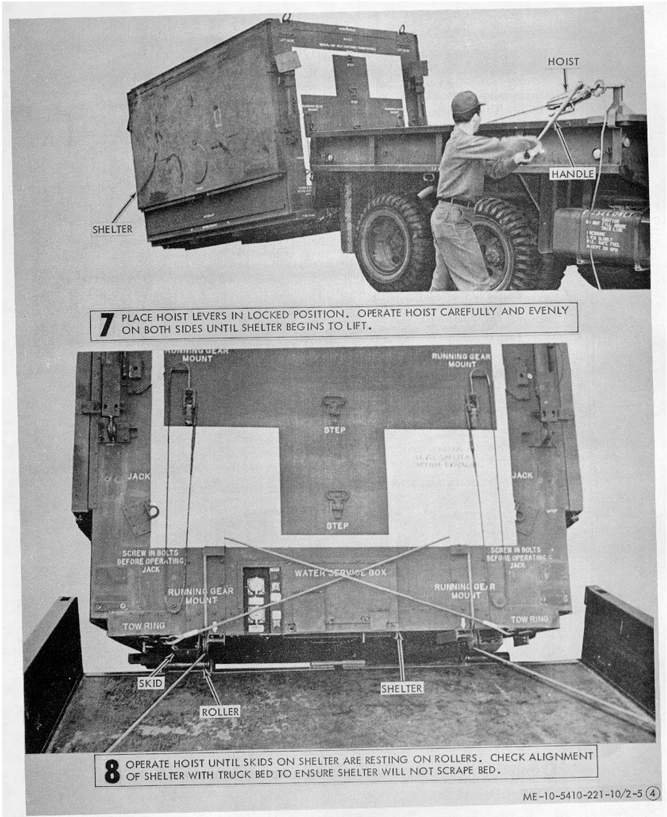
Figure 2-5(4). Loading expandable shelter on truck (sheet 4 of 6).
