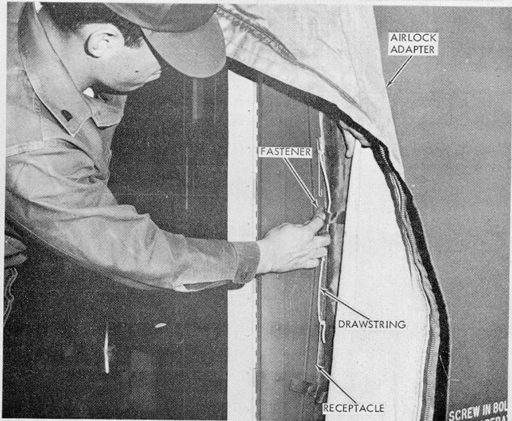
18 PRESS AIRLOCK ADAPTER INTO RECEPTACLE AND SECURE WITH FASTENERS. PULL DRAWSTRING TIGHT AND HOOK TO RECEPTACLE.
